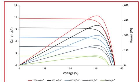
4) Average relative efficiency reduction of 5% at 200 W/m<sup>2</sup> according to EN 60904-1.
