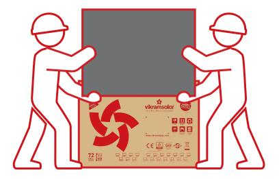
Fig 1: Correct way to unpack modules
