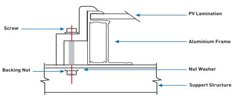
Fig 7: PV modules installed using fringe clamping method
