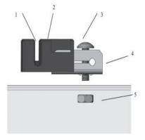
Fig 10: Grounding bolt # 1954381-2
