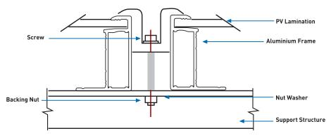
Fig 8: Middle modules installed using clamping method
