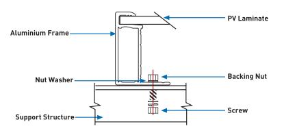
Fig 6: Modules Installed with Screw Fitting Method
